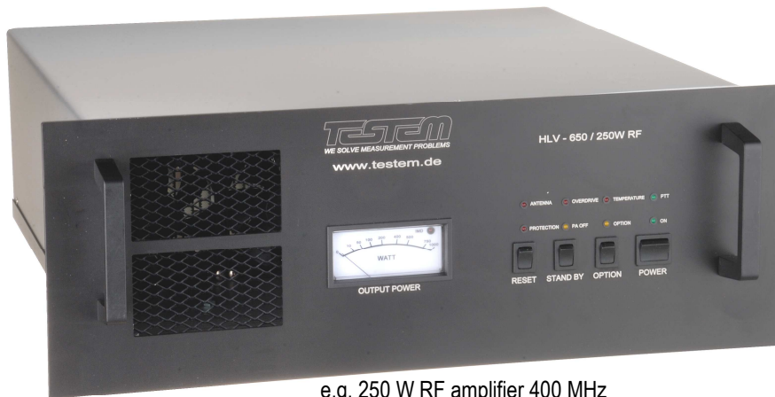
e.g. 250 W RF amplifier 400 MHz
